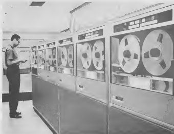
CHANGING TAPES on one of the six IBM 7330 tape units is N. van der Biesen, computer operator in the Electronic Data Processing and Computing Center. The information in a stack of IBM cards over 150 feet high can be stored in a single reel.
